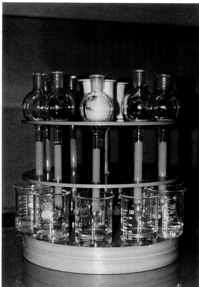
Fig. 3. First column with ion-exchange resin.
