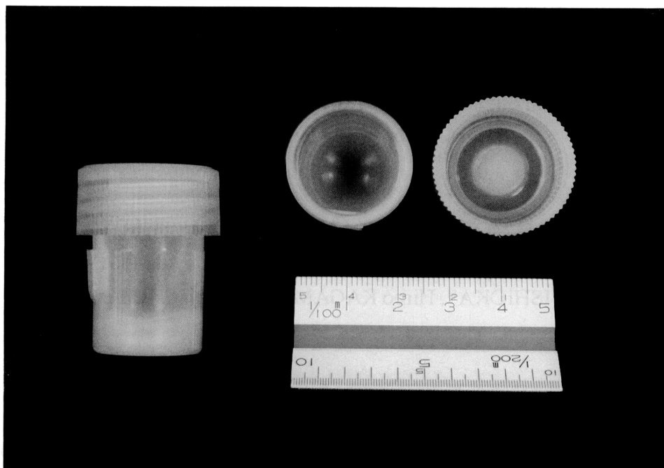
Fig. 1. Teflon vessel for decomposing rock powders. Capacity of this vessel is 7ml (scale bar is 5 cm).
