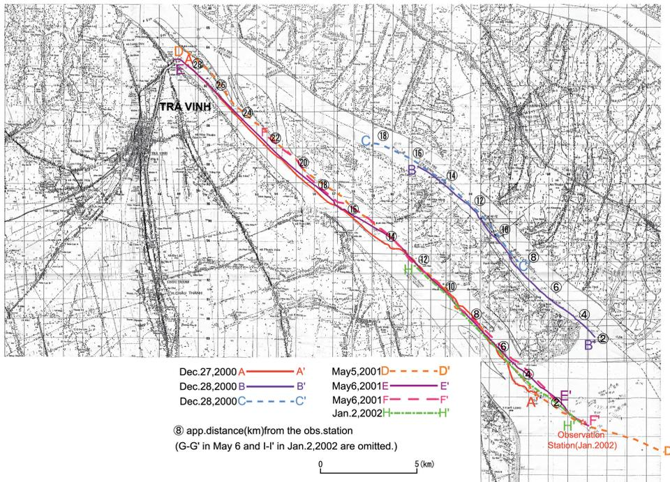
**Fig. 2.** The SC-3 echo sounding survey routes (routes G-G' of 6 May, 2001 and I-I' of 4 Jan., 2002 are omitted. These are roughly the same as routes F-F' and H-H', respectively. The topographic map is from the sheet 6228 Tra Vinh (1:100,000, Viet Nam).
