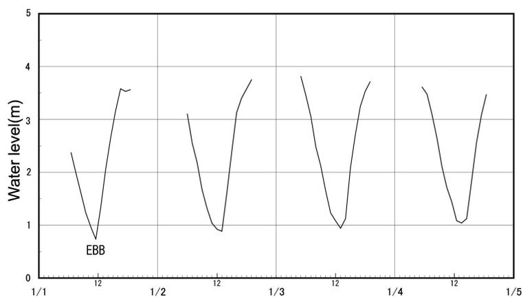
**Fig. 4.** Time-series plot of the water level at Tra Vinh Port (1 to 4 Jan., 2002)
