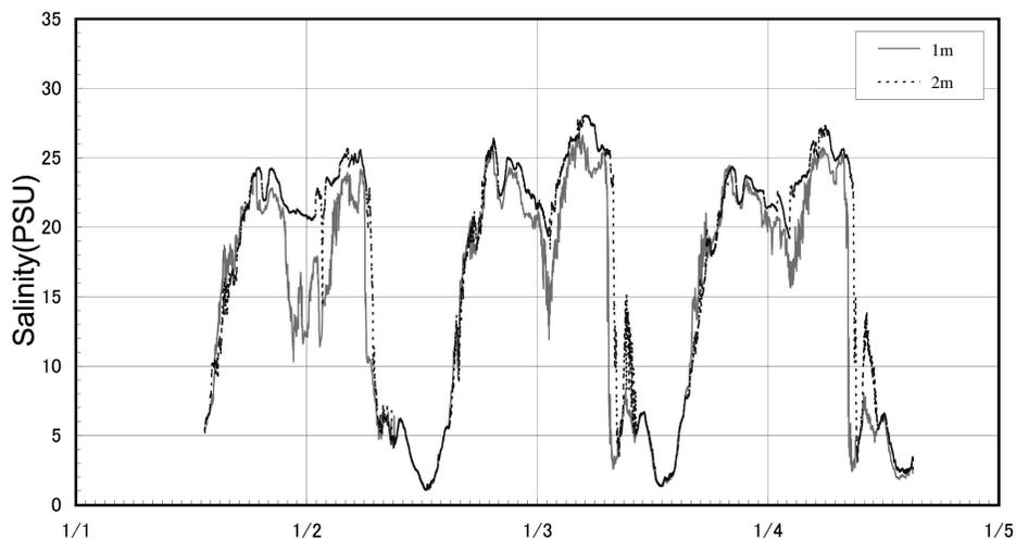
**Fig. 5.** Time-series plot of salinity at two horizons (1 and about 2 m depth in ebb tide ) at the river mouth observation station (1 to 4 Jan., 2002)
