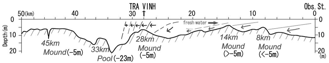
**Fig. 9.** Schematic profile of the Co Chien River and conceptual illustration of salt water intrusion in the intermediate and low flow seasons.
