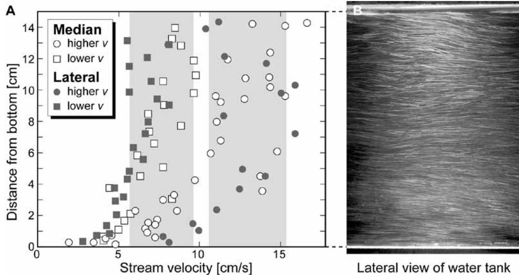
**Fig. 3.** Velocity distributions of median and lateral planes in the experimental area for two stream velocity conditions. **A.** Velocity distributions. Grey tones indicate stable intervals of velocities under the conditions of lower and higher stream velocities. **B.** Selected photograph of 0.05 s of a camera shutter opening showing the case of a median plane under the condition of a higher stream velocity. The photograph indicates that the stream was steady with no turbulent vortices.
