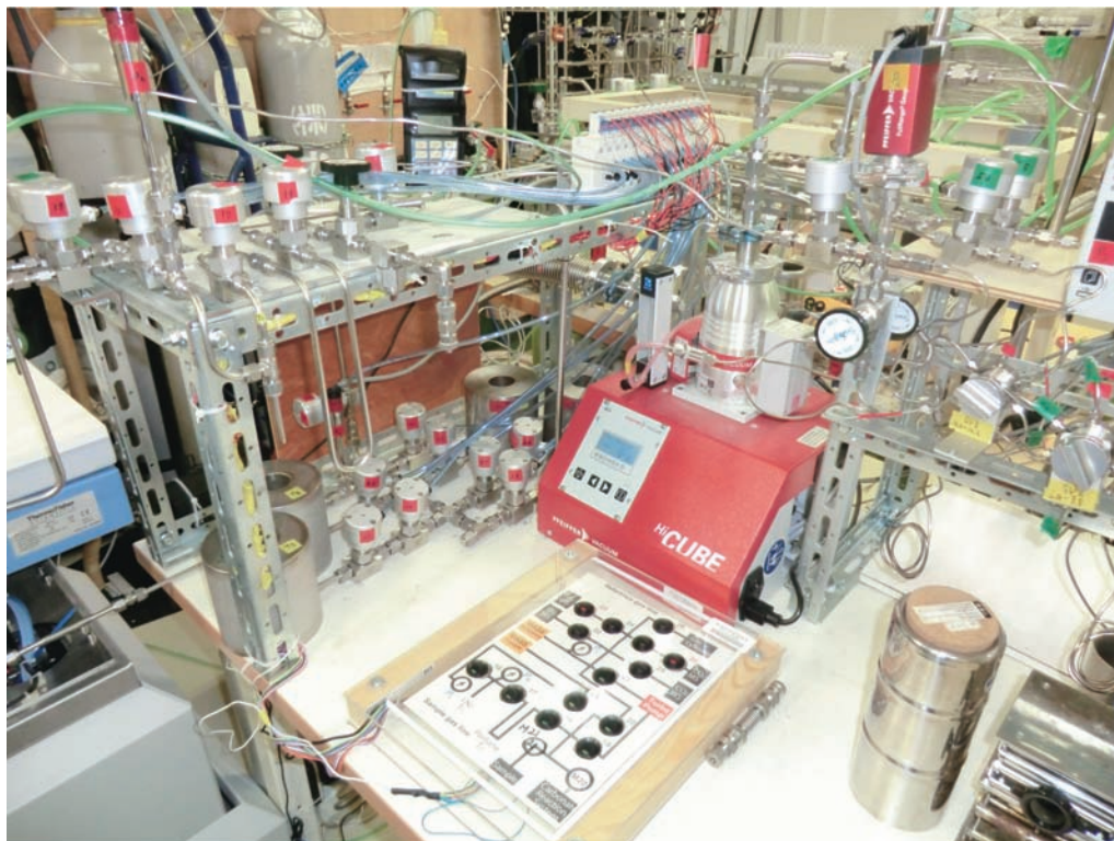
Fig. 5. A broad view of the inlet system for \text{CO}_2 and \text{SF}_6 standard gas and sample gas for carbon, oxygen and sulfur isotope analysis.
